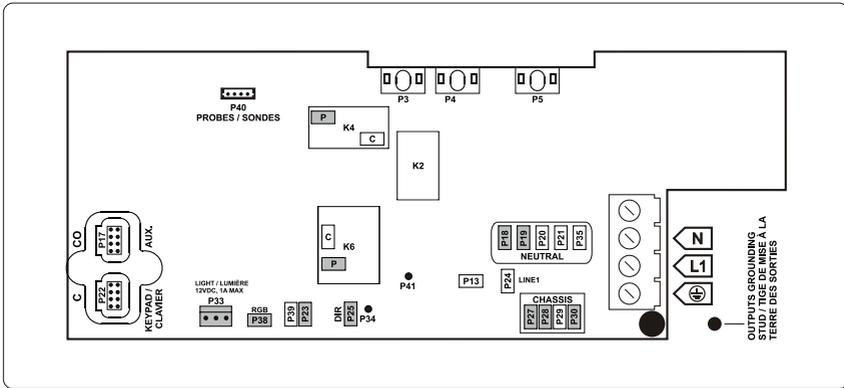
Make sure all accessories are linked to the bonding lug connector located on the side of the hot tub pack.
