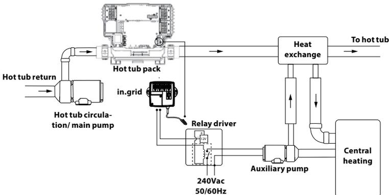
Please make sure your heat exchange does not have a flow restriction. The heater in your Y series hot tub control system needs a minimum of 20 GPM all the time.
