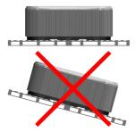
Ensure that your deck or foundation will support your hot tub. You must know the maximal load capacity of the foundation. Consult a qualified building contractor or structural engineer.
