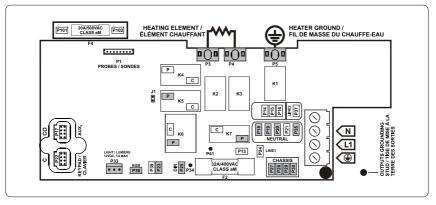
Make sure all accessories are linked to the bonding lug connector located on the side of the hot tub pack.
