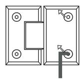
**18.1:** Remove the black rubber and make sure that the thick gray plastic is in place.
