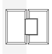
**18.4:** Place the cap on the back of the hinge and screw back on.
