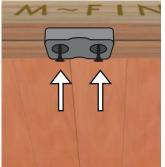
20.2: Assemble the large magnet to the flat piece.
