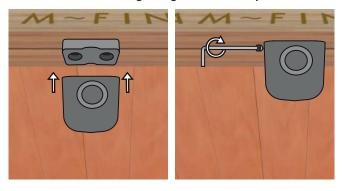
**20.3:** Use the special glass glue (included) to paste the oval shaped metal washer at the same height of the metallic door stop.
