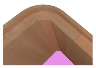
**4.5:** Join the ceiling to the walls and place the respective staples.
