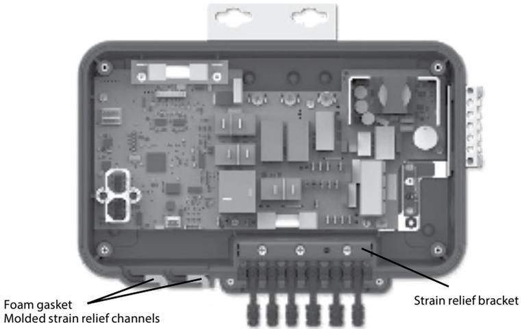
Once all low voltage cables are routed through the molded strain relief on the bottom of the spa pack, fill the remaining space with the foam gasket supplied.
