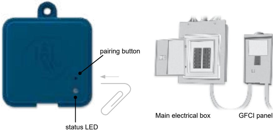
2. Press on the pairing button with a paper clip or some similar tool. When the pairing mode is active the status LED flashes YELLOW in a rapid pattern. The Home Transmitter is then in pairing mode and will remain in this mode until it pairs with an Spa Transmitter, or until it is reset (power cycled).
