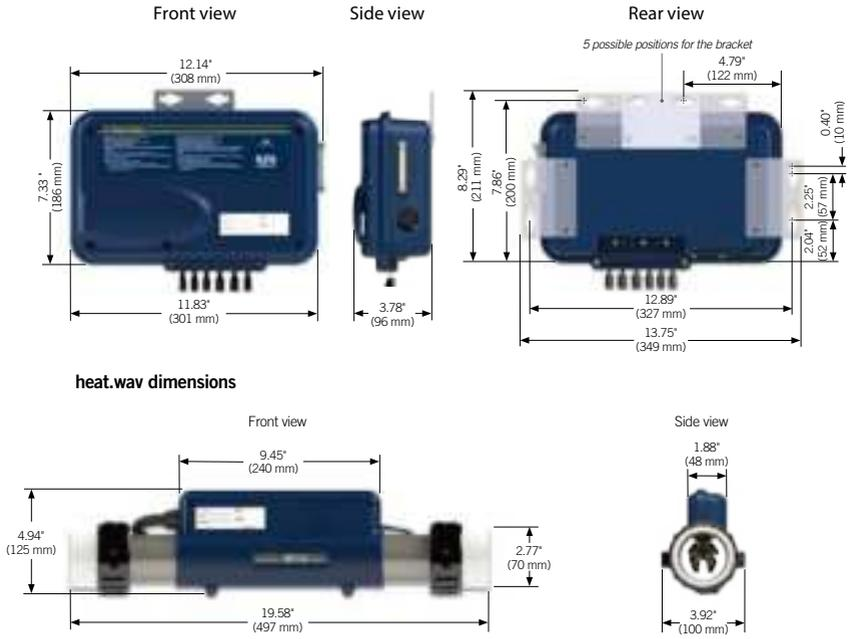
Note: Shown with optional wall mounting brackets (see Installation).
