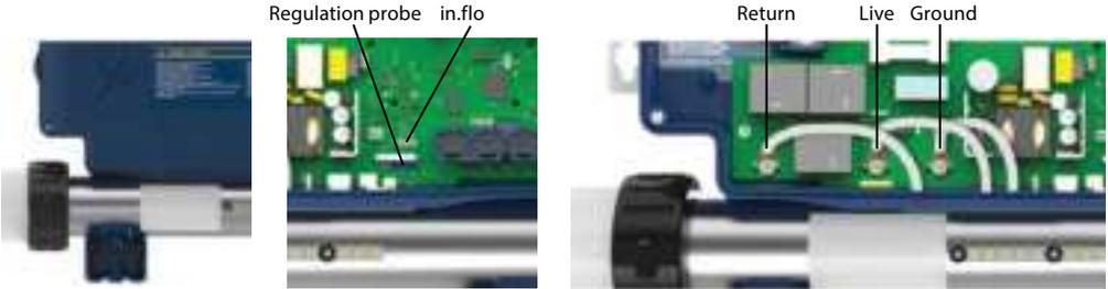
in.ye systems come with a high performance heat.wav heater. With no pressure switch, it features in.flo integrated dry-fire protection.
