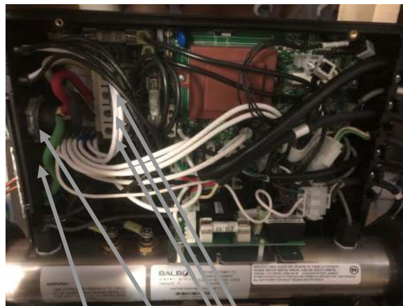
GROUND STRAIN RELIEF NEUTRAL LINE 1 LINE 2
