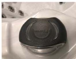
**Ultra Massage Selector: (Diverter Valve)** Located on swim spa lip this fitting is much larger than the air control described below. Turn to adjust pump power to selected jets which enhances water action through those jets by decreasing water action through others. Be sure that no sand or particles are brought into the swim spa as they will cause the diverter to seize up. It is best to turn the diverter valve only when the pump is turned off.
