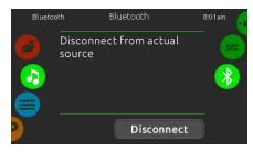
If a device with Bluetooth technology is connected to the in.stream 2, you can disconnect it by pressing the Disconnect key at the bottom of the
